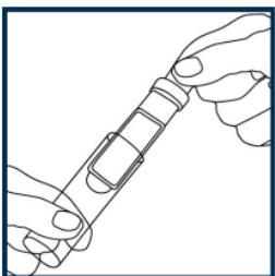
Remove the dipslide from the container by pulling the white tab while holding on to the outer cover.
