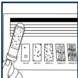
After incubation compare results of the dipslide to the dipslide comparison chart to quantify the results.
