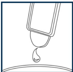
Excess fluid sample should be gently shaken from the paddle before it is placed back in to the container.
