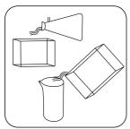
Rinse out vial with prepared Fill 50 mm vial with sample.
