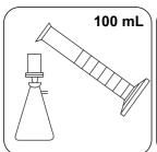
Filter approx. 100 mL sample with a pre-rinsed filter (pore size 0.45 µm).
