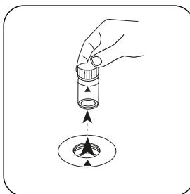
Remove the vial from the sample chamber.
