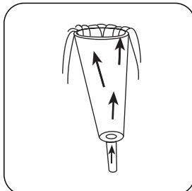
Run test water through the sampling vessel for several minutes from bottom to top to remove air bubbles.
