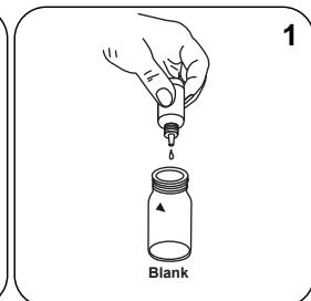
Place **1 drops** Vario **ALUMINIUM ECR Masking Reagent** in the blank.
