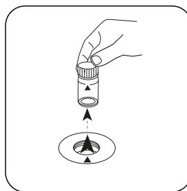
Remove the vial from the sample chamber.
