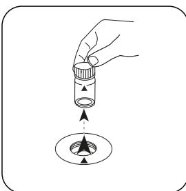
Remove the vial from the sample chamber.
