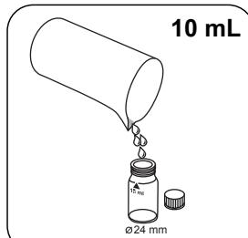
Fill 24 mm vial with **10 mL** prepared sample .
