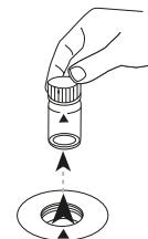
Remove the vial from the sample chamber.
