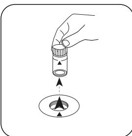
Remove the vial from the sample chamber.
