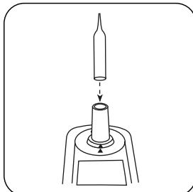
Place **Zero ampoule** in the sample chamber.
