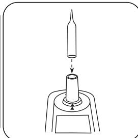
Remove zero ampoule from the sample chamber.
