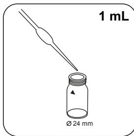
Place **1 mL (25 drops) Polyacrylate Buffer A1 solution** in the sample cuvette.
