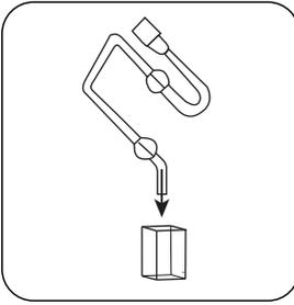
Fill 20 mm vial with the coloured absorption solution.
