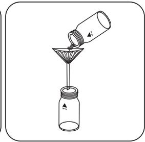
Any slight turbidity that occurs must be removed by filtration.
