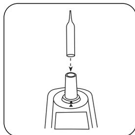
Place the ampoule in the sample chamber.
