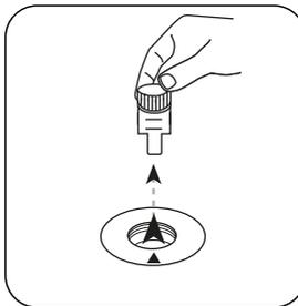
Remove **vial** from the sample chamber.
