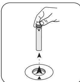
Remove **vial** from the sample chamber.
