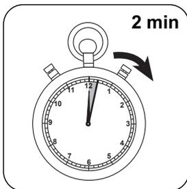
Wait for **2 minute(s) reaction time**. Press the **TEST (XD: START)** button. The result in mg/l Chloride appears on the display.
