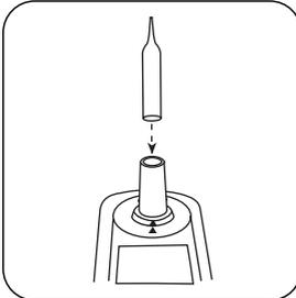
Place **Zero ampoule** in the sample chamber.
