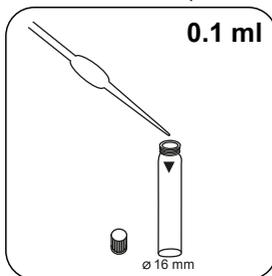
Add **0.1 ml (2 drops) Phosphate-101** to the digested sample.
