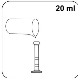
Put **20 ml sample** in 25 ml measuring cylinder
