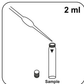
Fill sample vial with **2 ml prepared, digested sample.**
