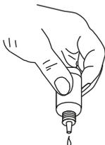
Hold cuvettes vertically and add equal drops by pressing slowly.
