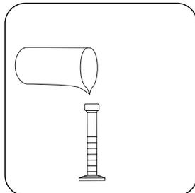
With the selected sample volume fill a 50 ml measuring cylinder. If necessary, fill up with demineralised water to 50 ml and mix.
