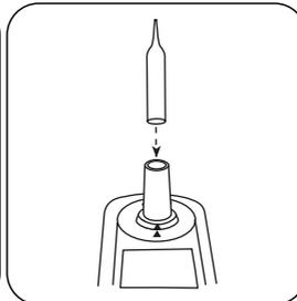
Place the ampoule in the sample chamber.
