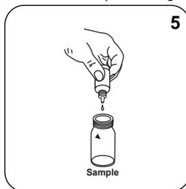
Add **5 drops Free Chlorine Reagent Solution** to the **sample vial**.
