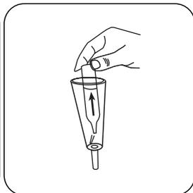
Then quickly remove the ampoule from the sampling vessel with the tip down.
