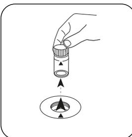
Remove the vial from the sample chamber.
