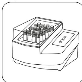
Warm vial for **120 minutes at 120 °C** in a pre-heated thermoreactor in **inverted position**.
