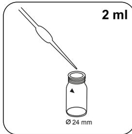
Put **2 ml sample** and **8 ml of deionised water** in the sample vessel.
