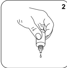
Add **2 drops KS135 (Phenolphthalein Substitute Indikator)**.
