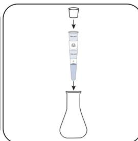
Close the absorption tubes with a plug and fit onto the Erlenmeyer flasks.
