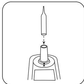
Place **Zero ampoule** in the sample chamber.
