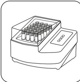
Seal the vials in the pre-heated thermoreactor for **120 minutes at 100 °C**.
