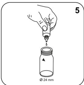
Add **5 drops Free Chlorine Reagent Solution** to the **vial**.
