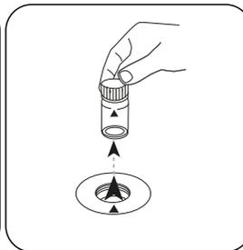
Remove the vial from the sample chamber.
