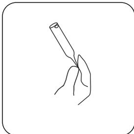
Close the opening with one finger, to avoid contact with the air.
