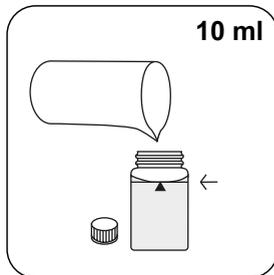
Fill Fluorescein mm vial with **10 ml sample**.
