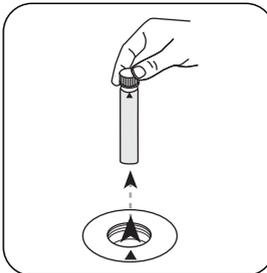
Remove **vial** from the sample chamber.
