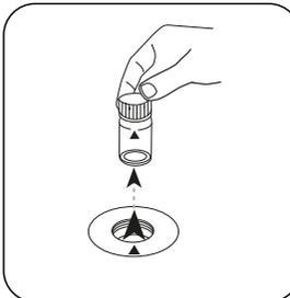
Remove the vial from the sample chamber.
