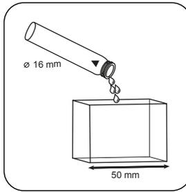
Fill 50 mm vial with prepared sample.
