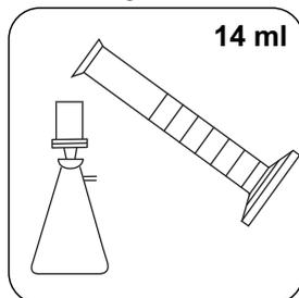
Filter approx. 14 ml sample with a pre-rinsed filter (pore size 0.45 µm).
