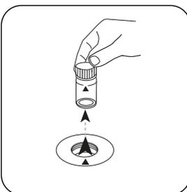
Remove the vial from the sample chamber.
