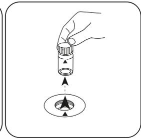
Remove the vial from the sample chamber.
