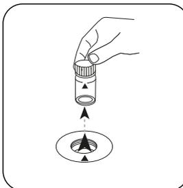
Remove the vial from the sample chamber.
