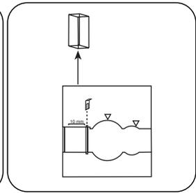
Remove **vial** from the sample chamber.
