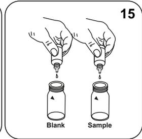
Add **15 drops Vario Molybdate 3 Reagenz-solution** to each vial.
