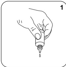
Add **1 drop KS135 (Phenolphthalein Substitute Indicator)**.
