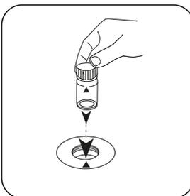
Place Chloramine vial in the sample chamber. • Pay attention to the positioning.
