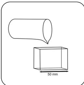
Fill 50 mm vial with prepared sample.
