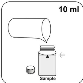
Fill sample vial with **10 ml prepared, digested sample**.
