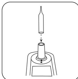
Remove zero ampoule from the sample chamber.
