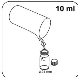
Fill 24 mm vial with **10 ml prepared sample**.
