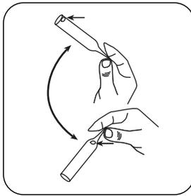
Invert the ampoule several times, allowing the bubble to move from one end to the other. Dry the outside.
