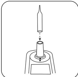
Place **Zero ampoule** in the sample chamber.
