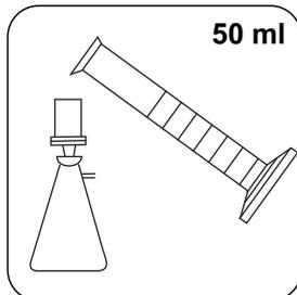
Filter approx. 50 ml sample with a pre-rinsed filter (pore size 0.45 µm).
