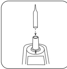
Place the ampoule in the sample chamber.
