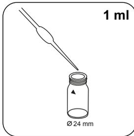
Place **1 ml (25 Tropfen) KS256 (Polyacrylate Reagenz 2) solution** in the test vial.
