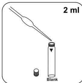
Place **2 ml of digested, pre-prepared zero sample** in the blank.
