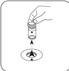
Remove the vial from the sample chamber.
