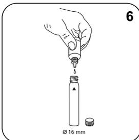
Add **6 drops H<sub>2</sub>O<sub>2</sub>-Reagent Solution**.
