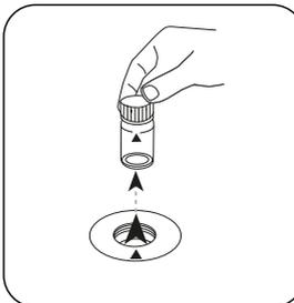
Remove the vial from the sample chamber.
