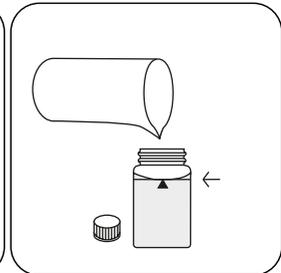
Fill up vial with **sample** to the **10 ml mark**.
