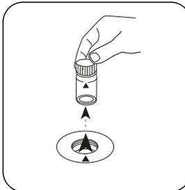
Remove the vial from the sample chamber.
