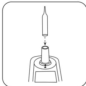
Place **Zero ampoule** in the sample chamber.
