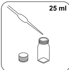
Fill one of the digestion vials with **25 ml of prepared sample**.
