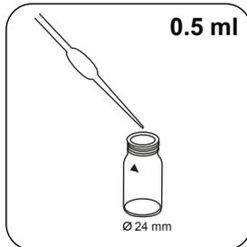
Place **0.5 ml Molybdenum 2 LR solution** in the test vial.
