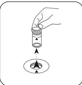
Remove the vial from the sample chamber.
