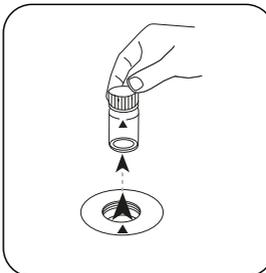
Remove the vial from the sample chamber.
