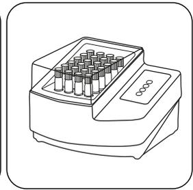
Seal the vials in the pre-heated thermoreactor for **120 minutes at 150 °C**.
