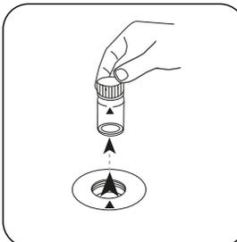
Remove the vial from the sample chamber.
