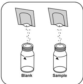
Add a **Monochlor FRGT powder pack** simultaneously in each vial.
