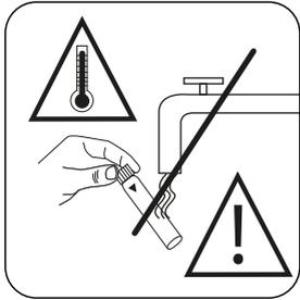
Allow vial to stand inverted for 1 hour and to cool. **Do not cool it with water!** After cooling down, rotate it and measure in the photometer **within 10 min**.
