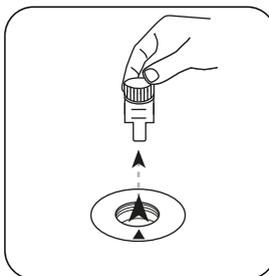
Remove **vial** from the sample chamber.
