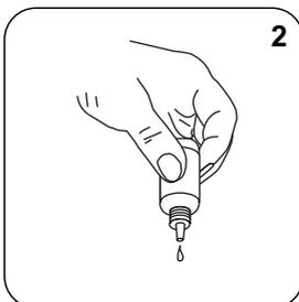
Add **2 drops KS135 (Phenolphthalein Substitute Indikator)**.
