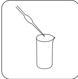
In the sample vessel, put **2 ml sample and 8 ml deionised water**.
