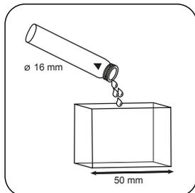
Fill 50 mm vial with prepared sample.
