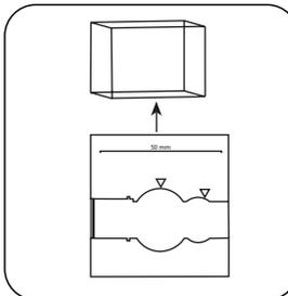
Remove **vial** from the sample chamber.
