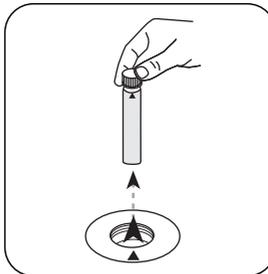
Remove **vial** from the sample chamber.
