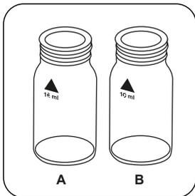
Prepare two clean 24 mm vials. Mark one as Chloramine and the other as Chlorine vial.
