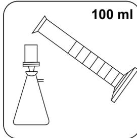
Filter approx. 100 ml sample with a pre-rinsed filter (pore size 0.45 µm).
