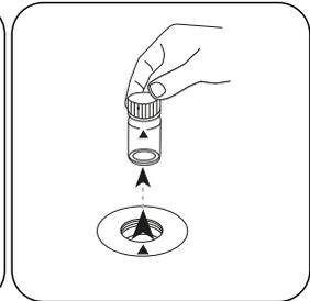
Remove the vial from the sample chamber.
