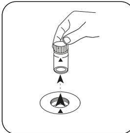
Remove the vial from the sample chamber.
