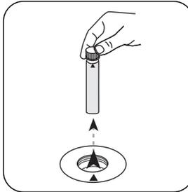
Remove **vial** from the sample chamber.
