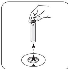
Remove **vial** from the sample chamber.
