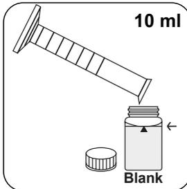
Fill blank with **10 ml prepared sample**.
