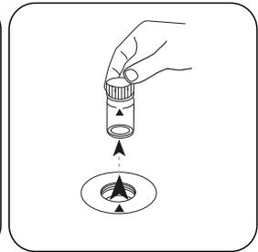
Remove the vial from the sample chamber.
