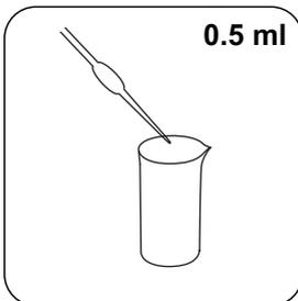
Place **0.5 ml Reagent Pb-1** in a suitable sample vessel.
