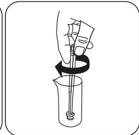
Crush tablet(s) by rotating slightly.
