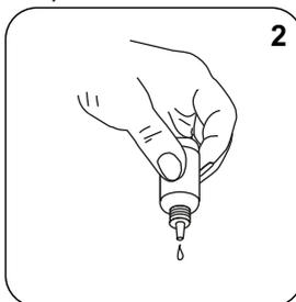
Add **2 drops KS135 (Phenolphthalein Substitute Indicator)**.
