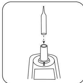
Remove zero ampoule from the sample chamber.
