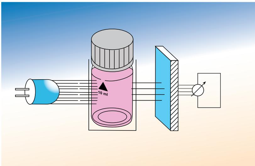
Transmission is the ratio of the intensity of light before ( $I_0$ ) and after ( $I$ ) radiating freely through the sample. To represent this absorption of light over a large area, a negative common logarithm of the transmission is usually chosen, which is also known as extinction or absorbency.
