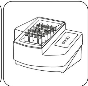
Seal the vials in the pre-heated thermoreactor for **60 minutes at 100 °C**.
