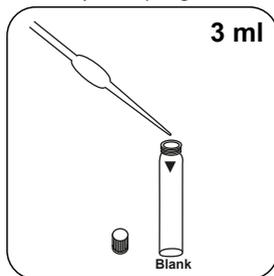
Place **3 ml of prepared zero sample** in the blank.
