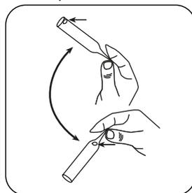
Invert the ampoule several times, allowing the bubble to move from one end to the other. Dry the outside.
