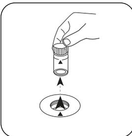
Remove the vial from the sample chamber.
