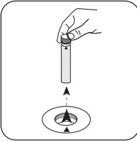
Remove **vial** from the sample chamber.
