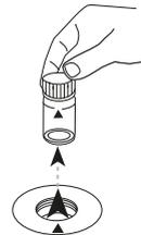
Remove the vial from the sample chamber.
