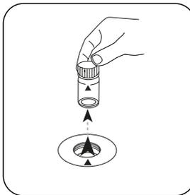
Remove the vial from the sample chamber.
