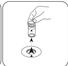
Remove the vial from the sample chamber.
