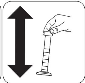
Stopper the mixing cylinder. Shake to dissolve the powder.
