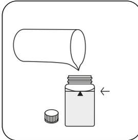
Fill up vial with **deionised water** to the **10 ml mark**.
