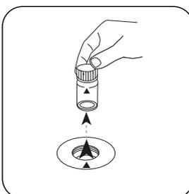
Remove the vial from the sample chamber.
