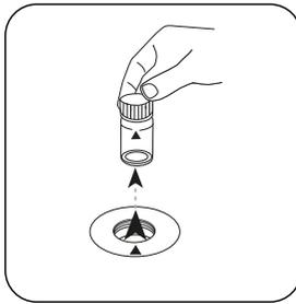
Remove the vial from the sample chamber.
