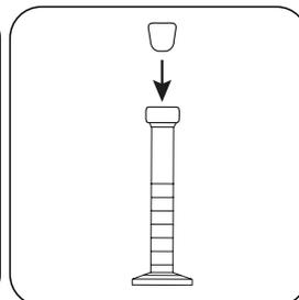
Stopper the mixing cylinder. Swirl around to dissolve the powder.
