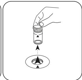
Remove the vial from the sample chamber.
