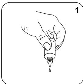
Add **1 drop KS135 (Phenolphthalein Substitute Indikator)**.
