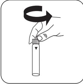
Open a digestion vial **PO<sub>4</sub>-P Acid Reagent**.
