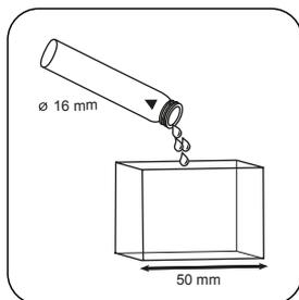
Fill 50 mm vial with prepared sample.
