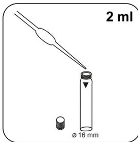
Add **2 ml 1,54 N Sodium Hydroxide Solution** to the digested sample.
