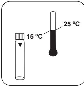
Allow the vial to cool to room temperature and then measure.
