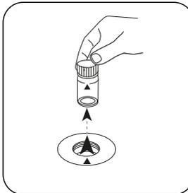
Remove the vial from the sample chamber.
