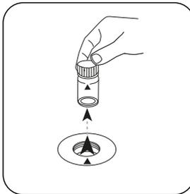
Remove the vial from the sample chamber.
