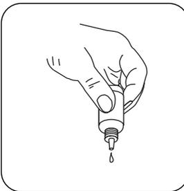
Add **KS 144 (Calcium Hardness Buffer)** drop by drop to the same sample until colouration turns from light pink to red. (**Note: make sure to swirl the vial after adding each drop!**)
