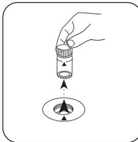
Remove the vial from the sample chamber.
