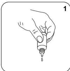
Add **1 drop KS135 (Phenolphthalein Substitute Indicator)**.
