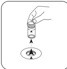
Remove the vial from the sample chamber.
