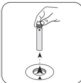
Remove **vial** from the sample chamber.
