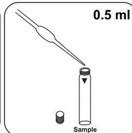
Fill sample vial with **0.5 ml prepared, digested sample**.
