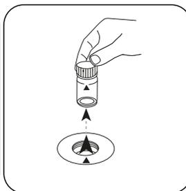
Remove the vial from the sample chamber.
