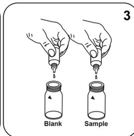
Add **3 drops Chloride-52 solution** to each vial.
