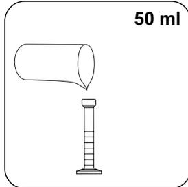
Put **50 ml sample** in 50 ml measuring cylinder
