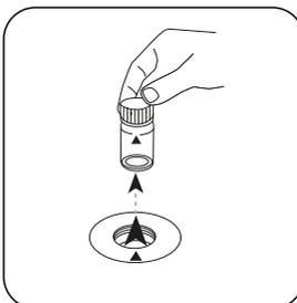
Remove the vial from the sample chamber.
