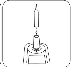
Remove zero ampoule from the sample chamber.
