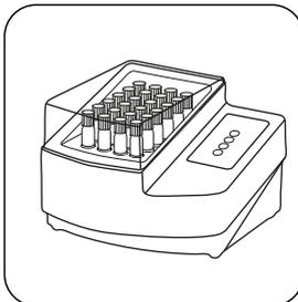
Seal the vials in the pre-heated thermoreactor for **30 minutes at 100 °C** .
