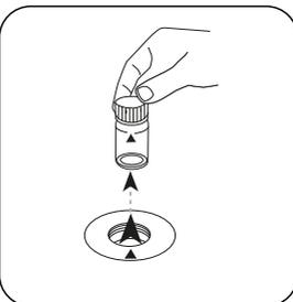
Remove the vial from the sample chamber.
