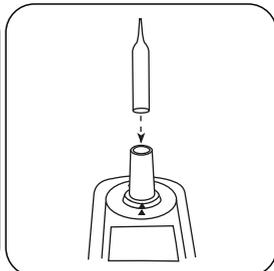
Remove zero ampoule from the sample chamber.
