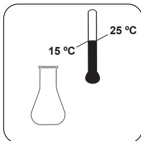
After the complete addition of the sulfuric acid, cool to room temperature in the ice bath.
