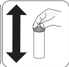
Close the test tube with the lid and mix the contents by vigorously shaking for 1 minute.
