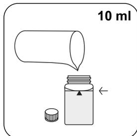
Place **10 ml Nitrite VHR L solution** in the test vial. Close vial(s).
