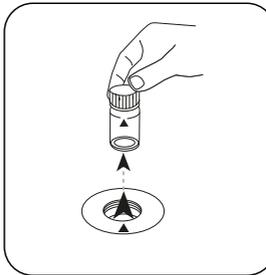
Remove the vial from the sample chamber.
