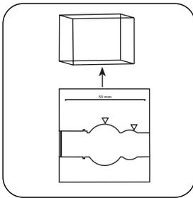
Remove **vial** from the sample chamber.
