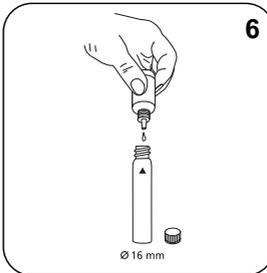
Add **6 drops H<sub>2</sub>O<sub>2</sub>-Reagent Solution**.
