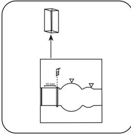
Remove **vial** from the sample chamber.
