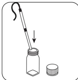
Keep the UV lamp in the sample. **Note: wear UV safety goggles!**
