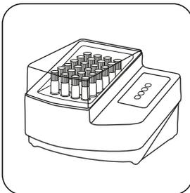
Seal the vials in the pre-heated thermoreactor for **120 minutes at 100 °C**.
