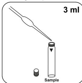
Place **3 ml of prepared sample** in the sample vial.
