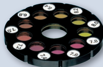
Test disc with colour stable glass standards
