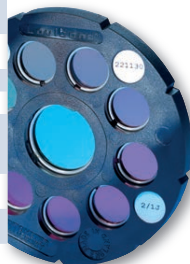
Test disc with colour-stable glass standards
