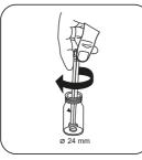
Crush tablet(s) by rotating slightly.
