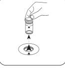
Remove the vial from the sample chamber.
