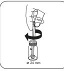
Crush tablet(s) by rotating slightly.
