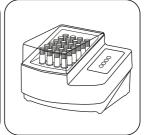
Seal the vials in the preheated thermoreactor for 120 minutes at 150 °C.
