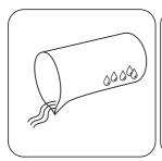
Rinse a beaker with the sample and empty it, leaving a few drops remaining in the beaker.
