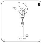
Add 6 drops H<sub>2</sub>O<sub>2</sub>-Reagent Solution.
