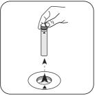
Remove **vial** from the sample chamber.
