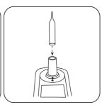
Place **Zero ampoule** in the Press the **ZERO** button. sample chamber.
