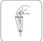
Then quickly remove the ampoule from the sampling vessel with the tip down.
