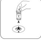
Remove the vial from the sample chamber.
