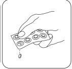
Add one DPD No. 1 tablet and one DPD No. 3 tablet straight from the foil into the first cleaned cuvette
