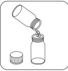
Fill prepared vial with prepared **glycine solution**.
