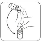
Dissolve tablet(s) by inverting.
