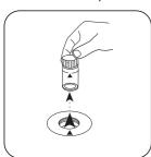
Remove the vial from the sample chamber.
