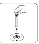
Remove vial from the sample chamber.
