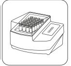
Seal the vials in the preheated thermoreactor for 30 minutes at 100 °C.
