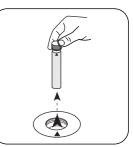
Remove **vial** from the sample chamber.
