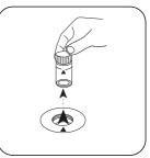
Remove the vial from the sample chamber.
