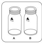
Prepare two clean 24 mm vials. Mark one as Chloramine and the other as Chlorine vial.
