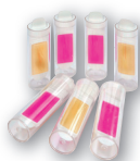
Dipslides for testing in Cooling Water
