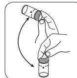
Dissolve tablet(s) by inverting.
