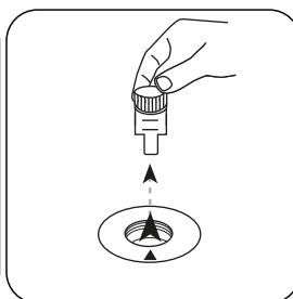
Remove **vial** from the sample chamber.
