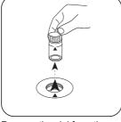
Remove the vial from the sample chamber.
