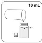
Fill 24 mm vial with 10 mL Close vial(s). sample.
