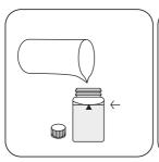
Fill up vial with sample to the 10 mL mark.
