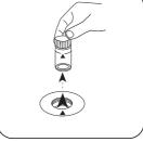
Remove the vial from the sample chamber.
