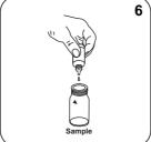
Add 6 drops DPD 1 Buffer Solution to the sample vial.
