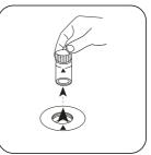
Remove the vial from the sample chamber.
