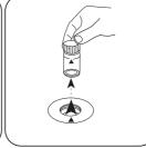
Remove the vial from the sample chamber.
