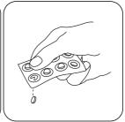
As an alternative to DPD No. 1 and No. 3 tablets, a DPD No. 4 tablet can be added.
