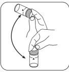
Dissolve tablet(s) by inverting.
