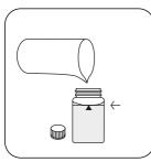
Fill up vial with **sample** to the **10 mL mark**.
