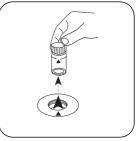
Remove the vial from the sample chamber.
