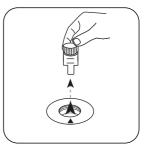
Remove vial from the sample chamber.
