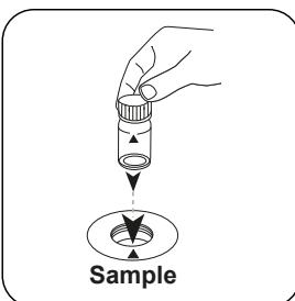
Place **sample vial** in the sample chamber. Pay attention to the positioning.
