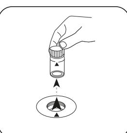
Remove the vial from the sample chamber.
