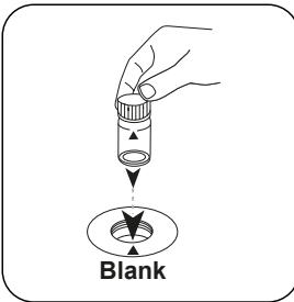
Place **blank** in the sample chamber. Pay attention to the positioning.
