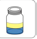
Allow phases to separate. A blue color should develop in the lower layer if any product is present.
