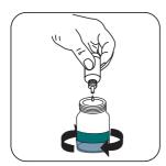
Add Polyamine Titrant P4/2 drop by drop to the sample until discolouration turns from blue to grey in the bottom layer (If P1/M layer is pink, the end point has been exceeded.).
