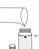
Fill up vial with **sample** to the **10 mL mark**.
