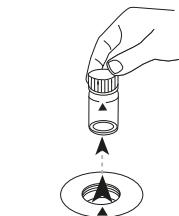
Remove the vial from the sample chamber.
