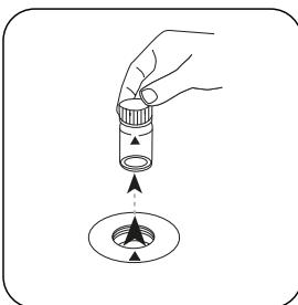
Remove the vial from the sample chamber.
