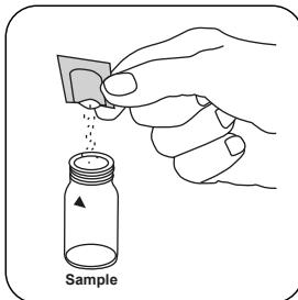
Adicionar à célula de amostra um **pacote de pó Vario Silica Amino Acid F10**.
