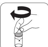
Place **sample vial** in the sample chamber. • Pay attention to the positioning.**Test**
