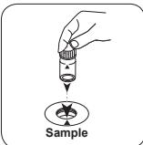
Place **sample vial** in the sample chamber. • Pay attention to the positioning.**Test**Press the **TEST (XD: START)** button.The result in Acid Capacity  $K_{S4.3}$  appears on the display.
