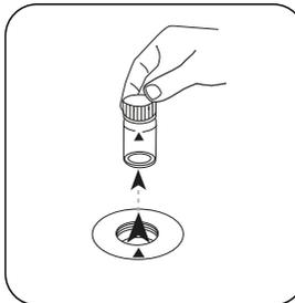
Remove the vial from the sample chamber.
