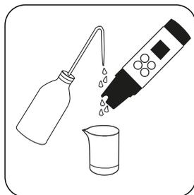
Rinse the electrode with distilled or deionised water and carefully wipe with a paper towel.
