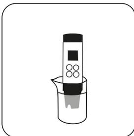
Hold the tester without protective cap in the sample water to be measured so that the electrode and temperature probe is immersed in the sample water not deeper than the seal ring.
