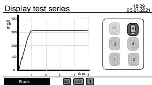
Use the head keys to select and deselect a sensor head to plot the measured data. A maximum of three plots can be displayed simultaneously for comparison.
