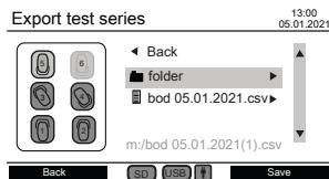
After selecting a storage medium, existing files and folders are displayed. Use the up ▲ and down ▼ arrow keys to select a folder or a file.
