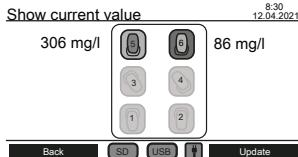
The latest measurements can be tracked in the submenu "Show current value". All six bottle positions are displayed in the center of the screen. The latest value is displayed next to the sensor head if connected to the system.
