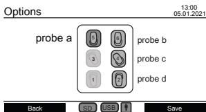
Enter the setting "Name heads" under "Options" to give the sensor heads a name. All six bottle positions are displayed in the center of the screen. The head keys can be used to select a bottle position. The bottle selection can be tracked by a red LED on the top of the sensor head. Use the number keys, the backspace key and the left ▲ and right ▼ arrow keys to enter a name for a selected sensor head.
