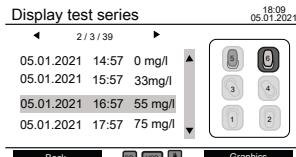
A schematic diagram of all bottle positions is displayed on the right side of the screen. The head keys can be used to select a bottle position. After, the measured data of the selected head are listed in mg/l with time stamp.
