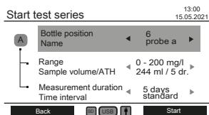
After sample preparation, enter the submenu "Start test series" to begin a measurement.
