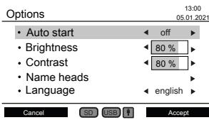
Instrument settings can be changed in the "Options" submenu. Use the up ▲ and down ▼ arrow keys to select a setting. Use the left ▲ and right ▶ arrow keys to change the selected setting. Use function key F2 to accept the new settings or function key F1 to return to the main menu.
