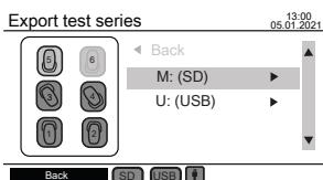
A schematic diagram of all bottle positions is displayed on the left side of the screen. Use the head keys to select and deselect the sensor heads for data export. Only selected heads are considered for data export. Use the up ▲ and down ▼ arrow keys to select between SD-Card and USB-drive if both are connected. Use the right ► arrow keys to continue with the data export.
