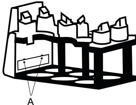
Remove all bottles from the rack in order to insert the batteries. Open the battery compartment (**A**) and insert three size C alkali-manganese cells (LR14 / 'baby cell') in the tubes provided for this purpose. The tube makes it easier to insert the batteries and prevent the batteries from jumping out again when you attempt to close the compartment.
