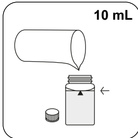
Fill 24 mm vial with 10 mL deionised water .
