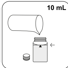
Fill 24 mm vial with 10 mL sample .
