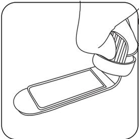
Sampling Surfaces: The sample should be taken by allowing direct contact between the agar surface and the test material. The paddle is flexible and can be bent at the upper end to allow both surfaces to come into intimate contact.
