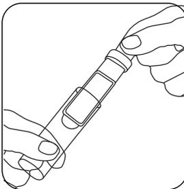
Place the dip slide back into the container while holding on the outer cover.
