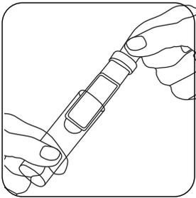
Remove the dip slide from the container by pulling the white tap while holding on to the outer cover.
