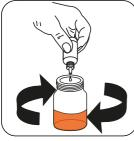
Add Chloride LR Titrant CC2 or Chloride HR Titrant BC2 drop by drop to the sample until colouration turns from yellow to orange/brown.
