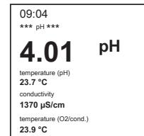
The pH value can be read in operating mode. Stop stirring while doing this.
