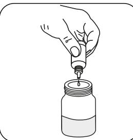
Add 4 drops of **Hardness Calcium Buffer CH2** per 10 mL of sample.
