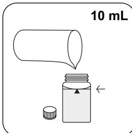
Fill 24 mm vial with **10 mL sample**. Close vial(s).
