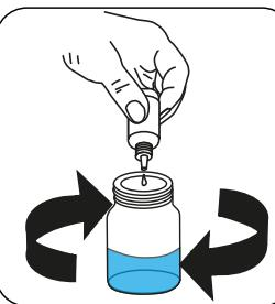
Add **Sulphite Titrant S2** drop by drop to the sample until colouration turns from colourless to blue.
