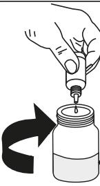
Add **Alkalinity LR Titrant TA3 or Alkalinity HR Titrant PA2/TA2** drop by drop to the sample until discolouration turns from **pink** to **colourless**.
