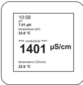
The measurement value can now be read off from the display. In the parameter configuration you can change the conductivity to TDS or salinity if required.
