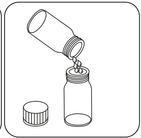
Fill prepared vial with prepared glycine solution .
