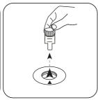
Remove **vial** from the sample chamber.
