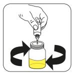
Add Alkalinity LR Titrant TA3 or Alkalinity HR Titrant PA2/TA2 drop by drop to the sample until colouration turns from purple to pale yellow.
