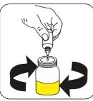
Add Alkalinity LR Titrant TA3 or Alkalinity HR Titrant PA2/TA2 drop by drop to the sample until colouration turns from purple to yellow.
