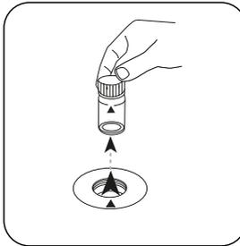
Remove the vial from the sample chamber.
