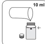
24-mm-Küvette mit **10 ml Probe** füllen.
