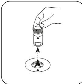
Remove the vial from the sample chamber.
