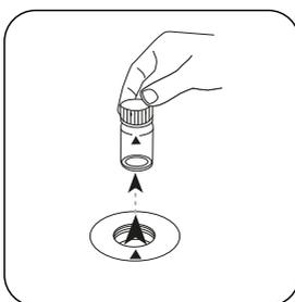
Remove the vial from the sample chamber.
