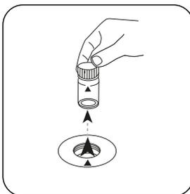
Remove the vial from the sample chamber.
