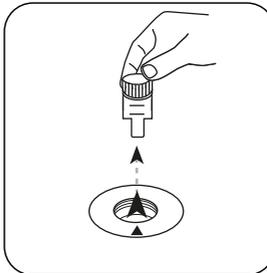
Remove **vial** from the sample chamber.
