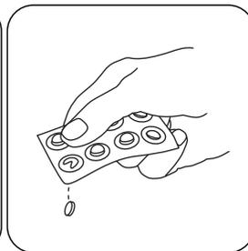
As an alternative to DPD No. 1 and No. 3 tablets, a DPD No. 4 tablet can be added.
