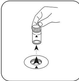
Remove the vial from the sample chamber.
