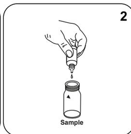
Add **2 drops DPD 1 Reagent Solution** to the sample vial.
