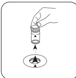
Remove the vial from the sample chamber.
