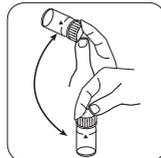
Dissolve tablet(s) by inverting.
