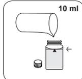
24-mm-Küvette mit **10 ml Probe** füllen.
