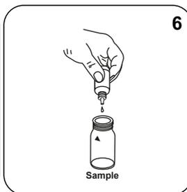
Add **6 drops DPD 1 Buffer Solution** to the sample vial.
