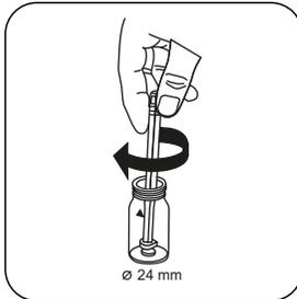
Crush tablet(s) by rotating
