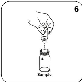
Add **6 drops DPD 1 Buffer Solution** to the **sample vial**.
