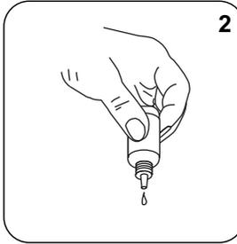
Adicionar **2 gotas KS135 (Phenolphthalein Substitute Indikator)**.
