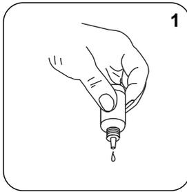
Adicionar **1 gota** **KS135 (Phenolphthalein Substitute Indikator)**.
