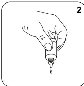
Adicionar **2 gotas KS135 (Phenolphthalein Substitute Indikator)**.
