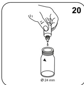
Adicionar **20 gotas KS253 (Chloride Reagent B)**.
