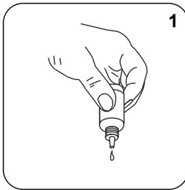
Adicionar **1 gota** **KS135 (Phenolphthalein Substitute Indikator)**.
