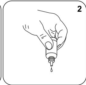
Adicionar **2 gotas KS135 (Phenolphthalein Substitute Indikator)**.
