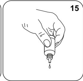
Adicionar **15 gotas KS278 (50% sulfuric acid)**.
