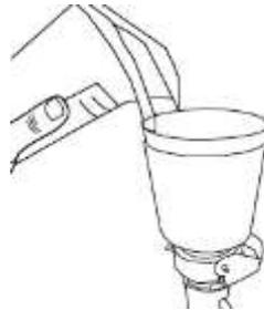
Pour sample into the filtration device
