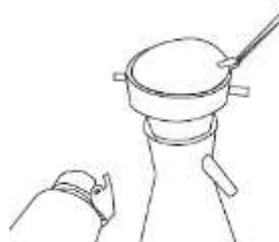
Place filter into filtration device
