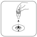
Remove **vial** from the sample chamber.
