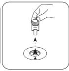
Remove **vial** from the sample chamber.
