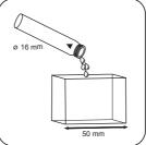
Fill 50 mm vial with prepared sample.
