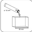
Fill 50 mm vial with prepared sample.
