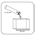
Fill 50 mm vial with prepared sample.
