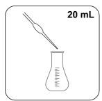
Put 20 mL homogenised sample in the erlenmeyer flask.
