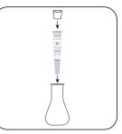
Close the absorption tubes with a plug and fit onto the Erlenmeyer flasks.
