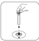
Remove **vial** from the sample chamber.
