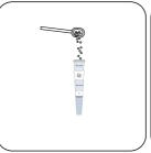
Add 6 - 7 g soda lime powder into the absorption tubes.
