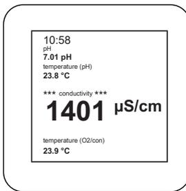
The measurement value can now be read off from the display. In the parameter configuration you can change the conductivity to TDS or salinity if required.
