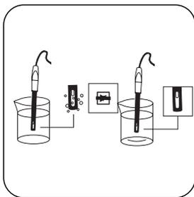
Immerse the measuring cell in the sample. During measurement, ensure that there are no air bubbles on the electrode surface and that the electrode, as well as the temperature sensor, are sufficiently surrounded by the sample.
