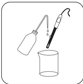
Rinse the electrode with distilled or deionised water and then with the sample.
