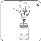
Add X drops of Nitrite Indicator N1 reagent to the sample, according to the selected sample volume (see table in the notes).
