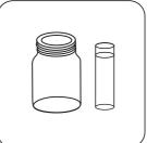
Use a titration jar for larger samples or test tube for smaller samples (5 mL or less).
