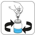
Add **Nitrite Titrant N2** drop by drop to the sample until colouration turns from **orange** to **blue**.
