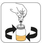
Add Zinc Titrant Z5 drop by drop to the sample until colouration turns from purple to pale orange.
