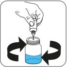
Add Hardness LR Titrant TH3 or Hardness HR Titrant TH4 drop by drop to the sample until colouration turns from wine red to blue.
