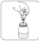
Add 4 drops of Hardness Total Buffer TH2 per 10 mL of sample.
