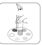
Look down through the tube, compare the colour produced in the tube to the colour standards printed on the comparison chart. Match to the nearest standard and read of the corresponding concentration value as Isothiazolinone in mg/l (ppm).
