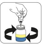
Add Anionics Titrant P9 or **Anionics HR Titrant P10** drop by drop to the sample until colouration turns from pink to blue.
